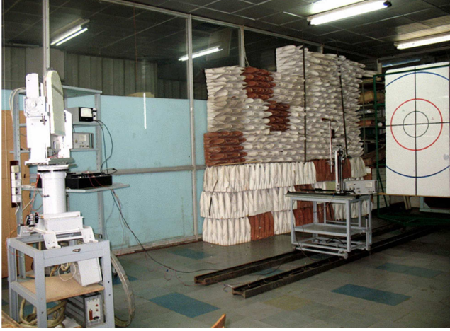
Figure 5. The main view of the experimental apparatus of the ADR's focused beam parameters measurements in conditions of laboratory premises.
